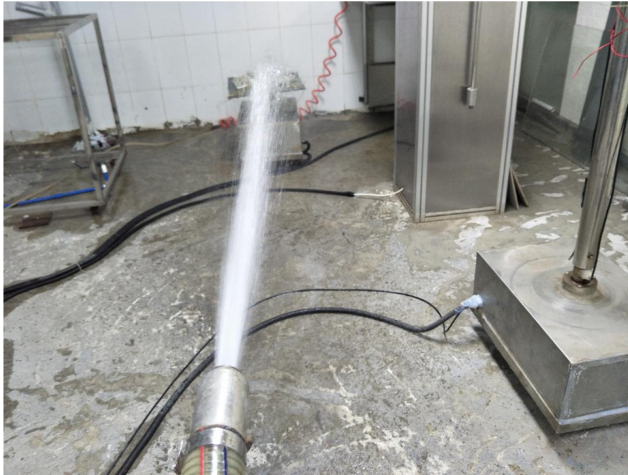
Photo 4: After IPX6 and IP6X test of model XNET180C
