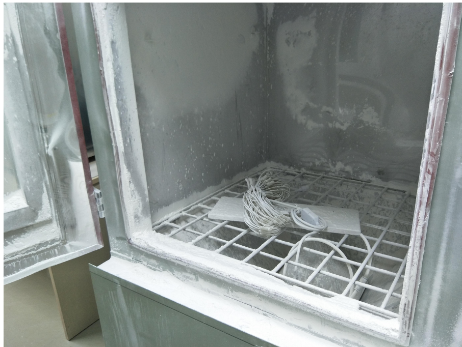
Photo 2: IP6X test of model XNET180C
