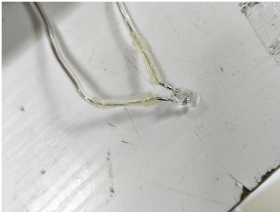
Photo 4: After IPX6 and IP6X test of model XNET180C
