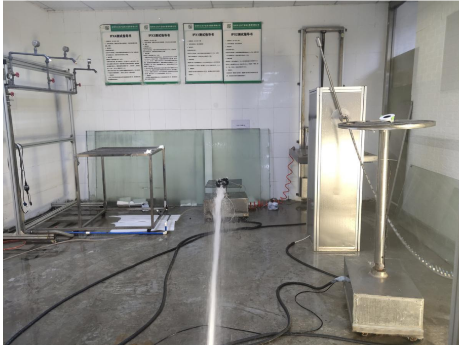
Photo 3: IPX5 test of model GLOBE
