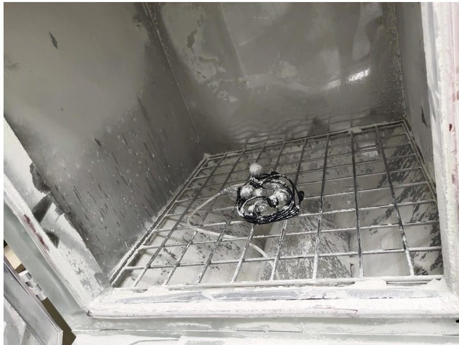
Photo 2: IP6X test of model GLOBE
