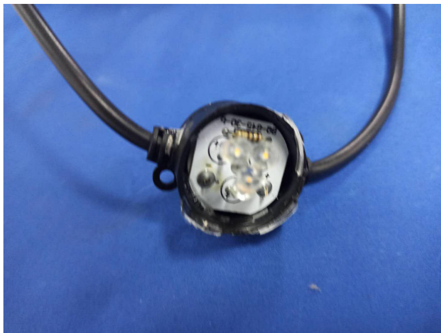
Photo 4: Test result after IP6X and IPX5 test
